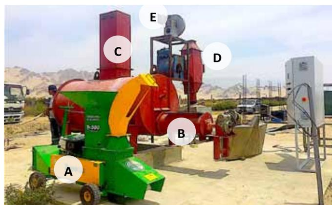
Figure 5. Integrated system from a pyrolyser of continuous production of fertilizers and spirulina. In the image the following phases are described (A) Biomass crusher, (B) entry of organic waste, (C) chimney for the conduction of gases, (D) exchanger for the recycling of heat for the drying of the microalgae and (E) use of CO<sub>2</sub> for the production of spirulina. Photo: Yngrid Espinoza.
